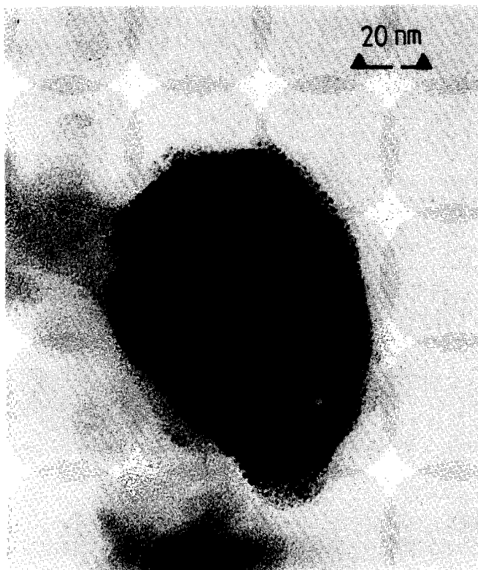
FIG. 7. Transmission electron micrograph of a Rh/SiO 2 slurry catalyst. Original magnification: 615,600 \times .
