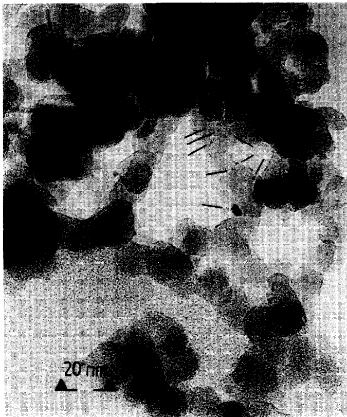
FIG. 5. Transmission electron micrograph of a very highly dispersed Rh/SiO 2 catalyst (catalyst 2 in Fig. 8 and 10). All rhodium appears in the form of two-dimensional rafts (—). Original magnification: 615,600 \times .
